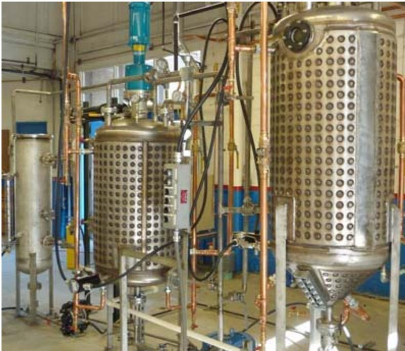
Northern's Biodiesel Testing Center has the new Biodiesel Pilot Plant finally installed at our campus; we have already made our first batch of biodiesel. Participants of the Biodiesel Workshop are "brewing" canola oil into biodiesel.
